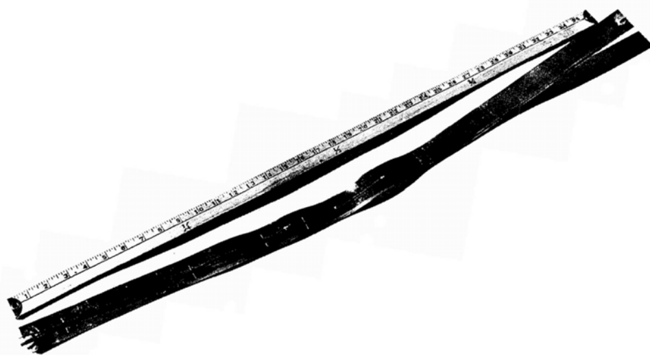
Figure 2-24: Bowed and Rippled Plate from the Spert III C-Core (Ref. 2-33)
