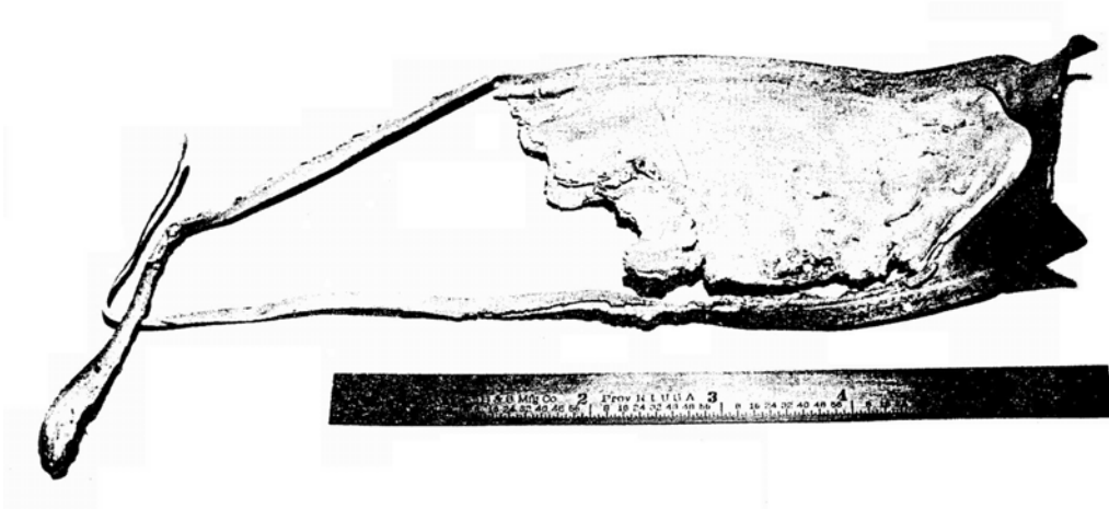
Figure 2-38: Recovered Fuel Plate from the Borax I D-test (Ref. 2-20)
