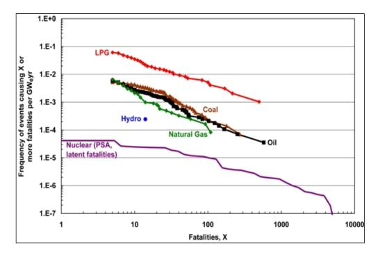
**Figure 2**: Comparison of frequency-consequence curves for full energy chains in OECD countries for the period 1969-2000. The curves for coal, oil, natural gas, LPG and Hydro are based on historical accidents and show immediate fatatlities. For the nuclear chain, the results originate from a plant-specific Probabilistic Safety Assessment (PSA) of a nuclear power plant and reflect latent fatalities.
