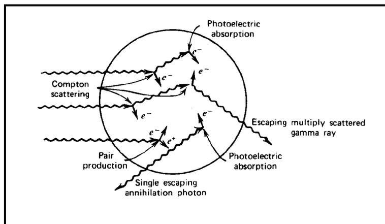
**Fig. 3: Intermediately sized detector**
