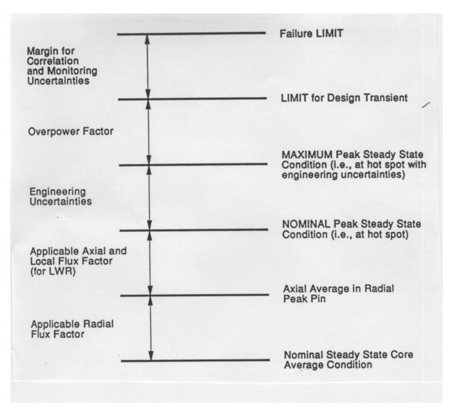
Figure 3.2: Thermal Design Margins
