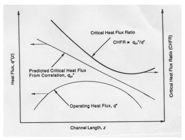
Figure 3.1: Critical Heat Flux Ratio
