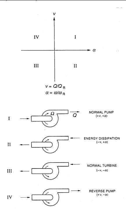
Figure 3.3: Pump Different Regimes of Operation
