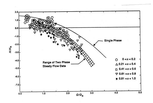
Figure 3.4: Pump Characteristics in Two-Phase Flow Operation
