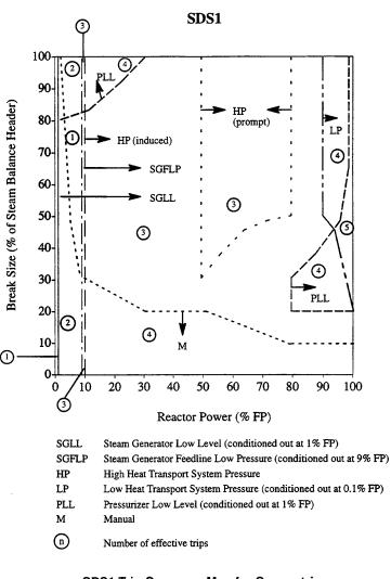
SDS1 Trip Coverage Map for Symmetric Steam Balance Header Breaks
