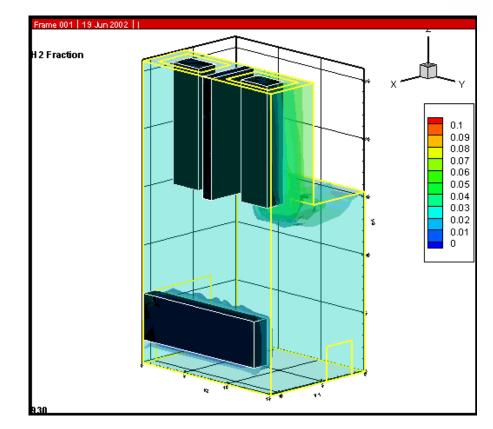
Predicted hydrogen distribution in containment during a large LOCA (header break).
