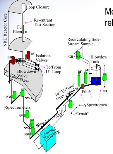
Measurement of CANDU fuel fission product release under severe accident conditions.
