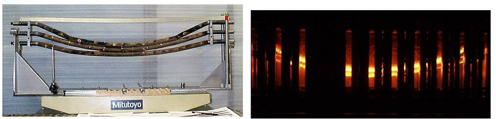
Tests with scaled arrays of CANDU fuel channels
