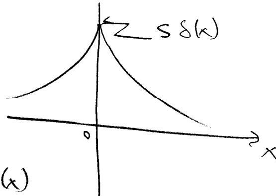
$$\therefore -D \frac{\partial^2 \phi}{\partial x^2} + \Sigma_a \phi = S \delta(x)$$
