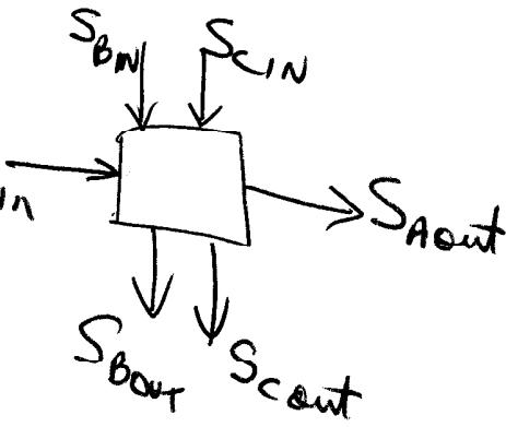
$$\frac{\partial N_B}{\partial t} = S_{B,in} - S_{B,out} + \sigma_A N_A \phi - \sigma_B N_B \phi - \lambda_B N_B \quad \left| \lambda_B = \frac{\ln 2}{T_L} \right.$$
