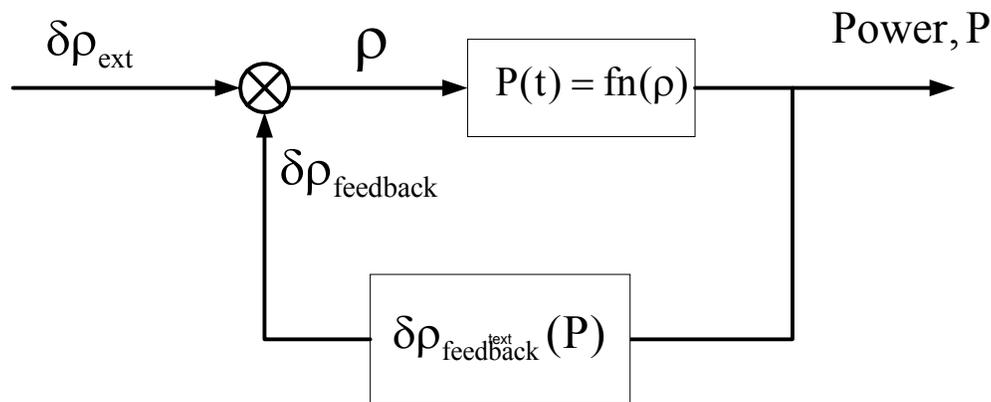
**Figure 2 Feedback loop for the power coefficient of reactivity**
