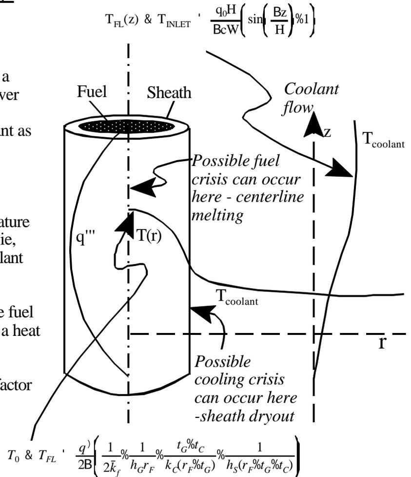
**Figure 5.1** Overview of fuel heat transfer
